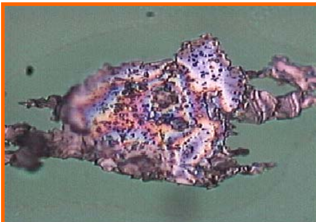
ROLLING CONTACT (Bearing) WEAR: Heat Tempered Particles applied to substrate by REO-1 Instrument
